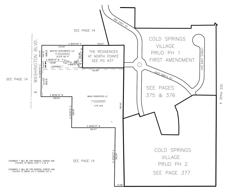
10' UTILITY & DRAINAGE EASEMENTS EACH SIDE OF PROPERTY LINES AS INDICATED BY DASHED LINES EXCEPT AS OTHERWISE SHOWN.
